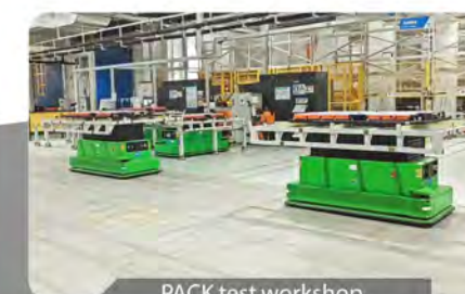
PACK test workshop intelligent transportation logistics system
